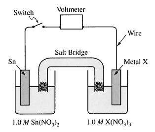
6. An electrochemical cell is constructed with an open switch, as shown in the diagram above. A strip of Sn and a strip of an unknown metal, X, are used as electrodes. When the switch is closed, the mass of the Sn electrode increases. The half-reactions are shown below.
