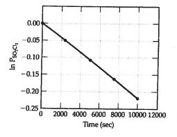
Graph In  $P_{SO_2Cl_2}$  vs. time. (Pressure is a satisfactory unit for a gas, since the concentration in moles/liter is proportional to P.) The graph is linear with slope  $-2.19 \times 10^{-5} \text{ s}^{-1}$  as shown on the figure. The rate constant  $k = -\text{slope} = 2.19 \times 10^{-5} \text{ s}^{-1}$ .
