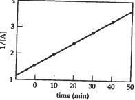
The plot of 1/[A] vs time is linear, so the reaction is second-order in [A].
