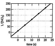
The plot of  $1/[NO_2]$  vs time is linear, so the reaction is second order in  $NO_2$ .
