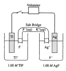
It is observed that when silver metal is placed in aqueous thallium(I) fluoride, TIF, no reaction occurs. When the switch is closed in the cell represented above, the voltage reading is +1.14 V.
